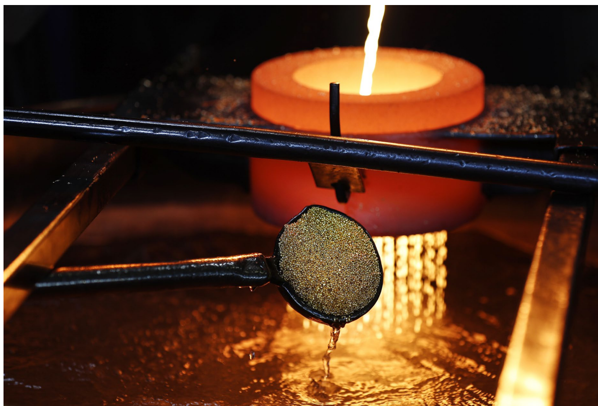
Gold casting grain is scooped in a metal ladle during the refining process © Bloomberg Creative Images/Getty Images
